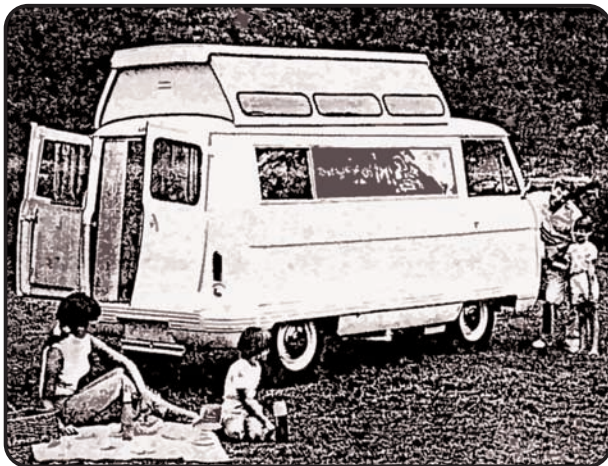
A Commer 'Wanderer' with novel 'Parkstone' design roof up, to give just over 6' clearance.
