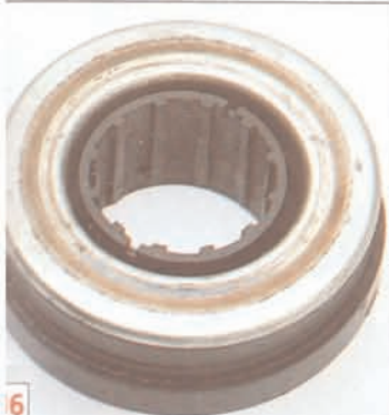
16 EXCESSIVE WEAR ON BEARING FACE See page 10.
