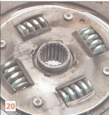
20 TORSION SPRINGS FOULING FLYWHEEL See page 10.
