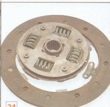
24 BROKEN DRIVEN PLATE CENTRE See page 16.
