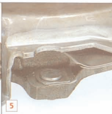
5 BROKEN DRIVE STRAPS See pages 4 and 14.
