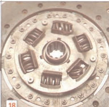
18 BROKEN TORSION SPRINGS See page 10.
