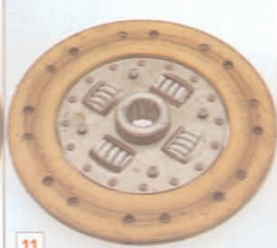
11 UNEVEN WEAR ON DRIVEN PLATE FACING See pages 6 and 12.
