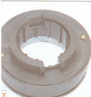
2 BROKEN CLIP ON RELEASE BEARING See page 14.
