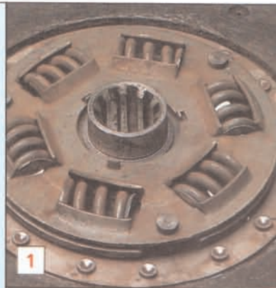
1 RUST ON DRIVEN PLATE See page 4.
