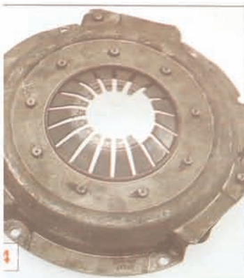
4 WORN DIAPHRAGM SPRING FINGERS See page 4.
