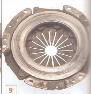
9 UNEVEN WEAR ON PRESSURE PLATE See page 6.
