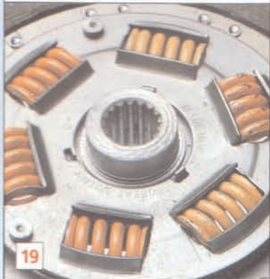
19 DAMAGED DRIVEN PLATE HUB See page 10.
